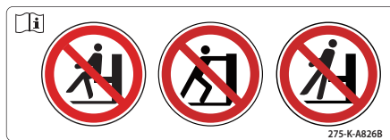
[Label 2. Prohibition of seating on control panel and "Tip-Over"]
