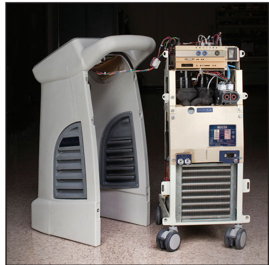
Fig. 8-13 Shell separated from internal components
