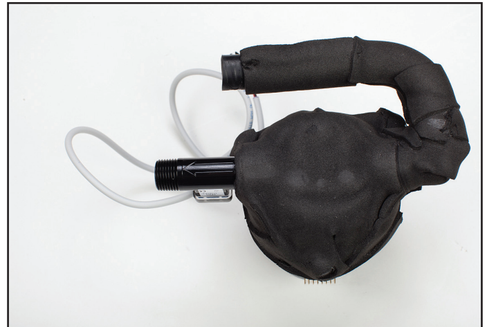
Fig. 8-50 Flowmeter with arrow indicating direction of flow; same direction as Circulation Pump output
