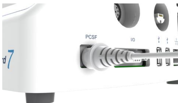
Figure 16: Connecting the tubing cable set to the LiquoGuard®7
