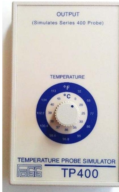
*Figure 11-10: Thermostat Verification Tool (P/N*
