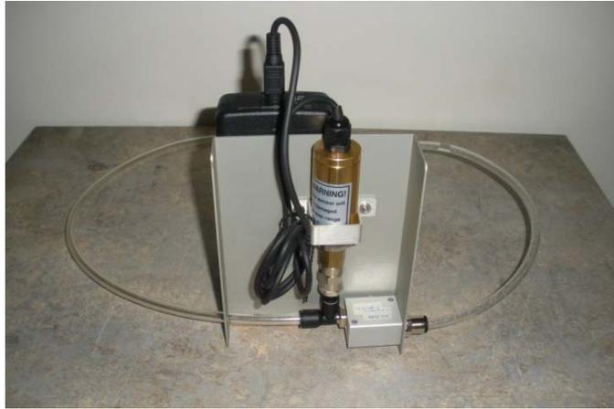
*Figure 11-6: Pressure Gauge connected*
