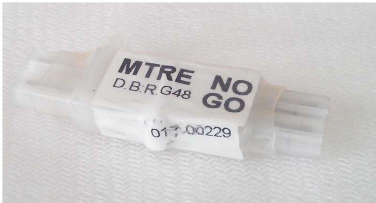
*Figure 9-2: Thermostat Verification Tool*
