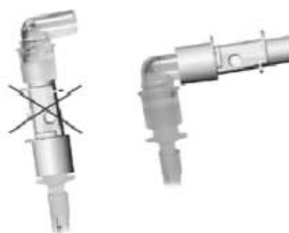
Figure 18: Incorrect and correct positioning of the airway adapter
