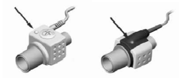
Figure 14: LED indicates if the sensor is ready for use
