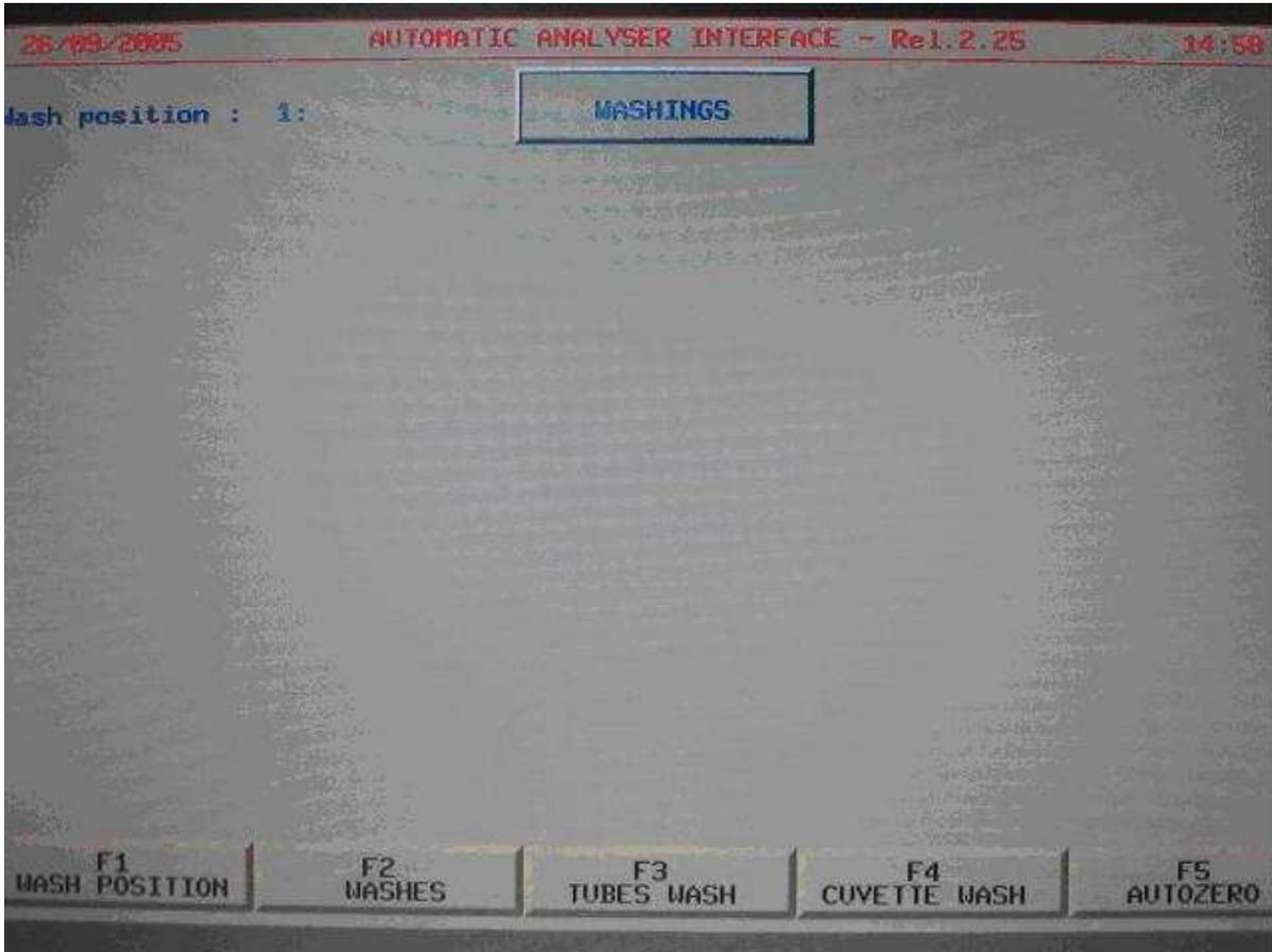
**F1 WASH POSITION** : Used to select the number of hole used for the wash ( on the example, the First hole on the first reaction segment )
