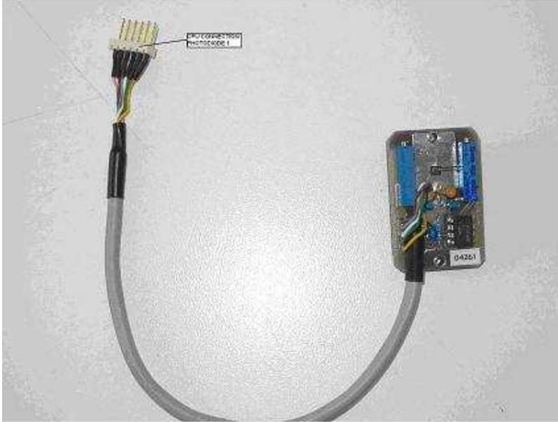
Figure 4: PREAMPLIFIER Board ( double cuvette )
