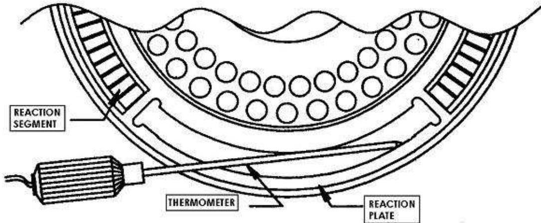
38) position a thermometer in the optical group inserting the end of it through the central hole of the false flow cell which should be inserted at the place of the true one in the optical group.
