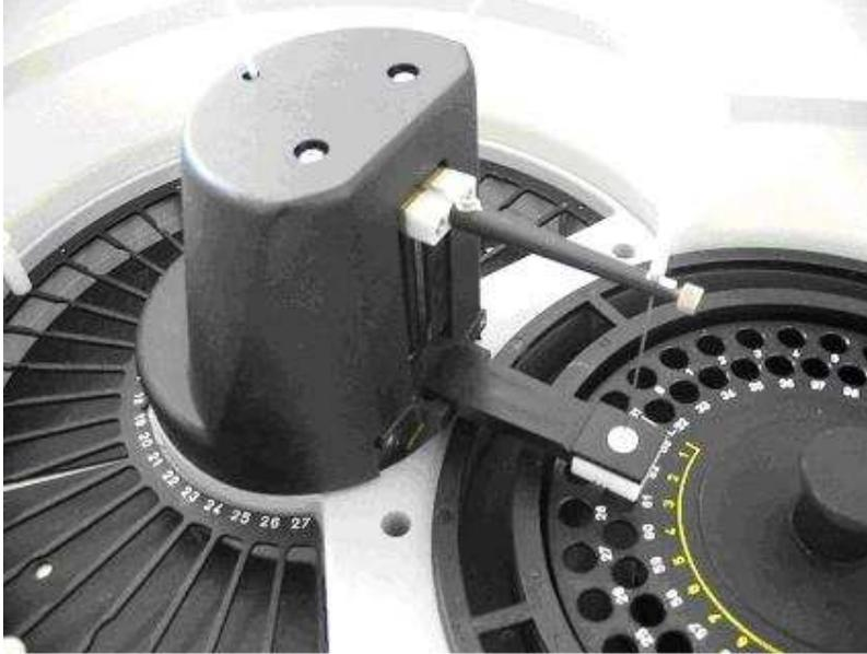
The sampling needle arm movement and position is controlled by a stepper motor driver (U12) located onboard to the Power board that drives the stepper motor model 103-546-5342 and an optical sensor barrel that informs when the arm is at home position. The movement from the motor to the arm is transferred by a mechanism driven from a belt and two pulleys.
