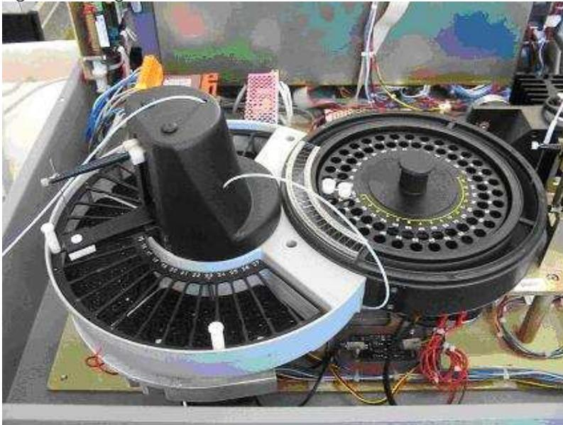
The Reagent plate movement and position is controlled by a stepper motor driver (U11) located onboard to the Power board that drives the stepper motor model 23L-C304-76W and an optical sensor barrel that informs when the arm is at home position. The movement from the motor to the arm is transferred by a mechanism driven from a belt and two pulleys.
