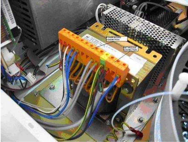
Select the main voltage on main transformer in order to connect the instrument to 115 VAC or 220 VAC.
