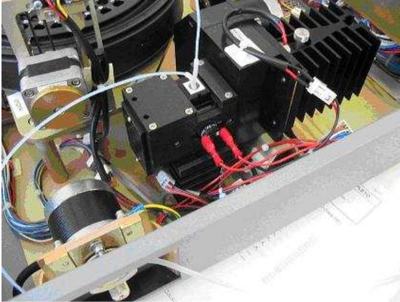
Figure 11: Optical group ( double cuvette )
