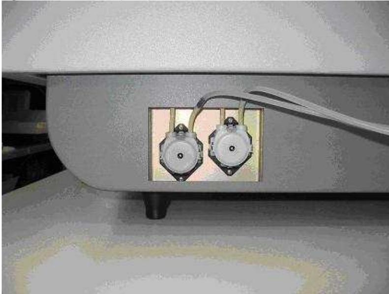
The PERISTALTIC PUMPS movement is powered directly from the Power board that drives two direct current motor 12 VCC ( ASF Thomas )
