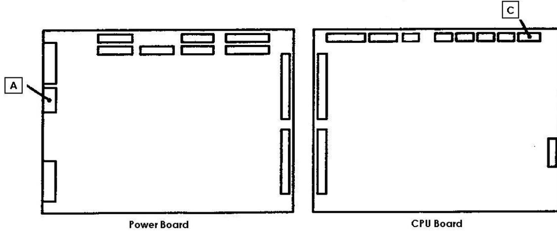
A = MX396 8 poles with the notes VID, V1, V2, L1 on the connector J2 of the power board
