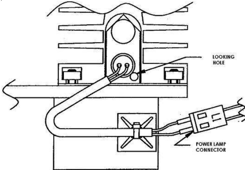
20) regulate the lamp tension connecting the tester on the two pin of the cabling connector L1 present near to the lamp itself, and regulate the trimmer P1 on the power board to obtain a value of the tension equal to  $+5,65 \text{ Vcc} \pm 0,05\text{V}$ .
