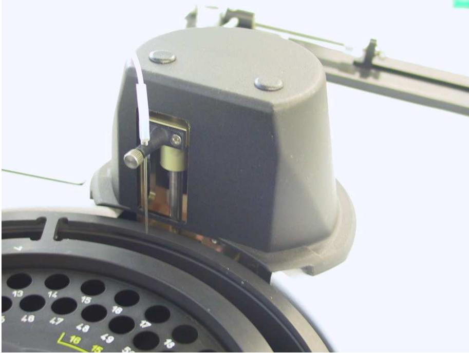
Figure 7: Aspiration Needle Arm ( double cuvette )
