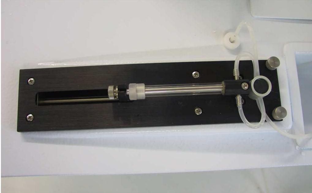
The SYRINGE movement and position is controlled by a stepper motor driver (U10) located onboard to the Power board that drives an stepper motor model HY200 1713 0100 and an optical sensor barrel that informs when the syringe is at home position. The movement from the motor to the syringe is made by a mechanism driven from a no-ending screw.
