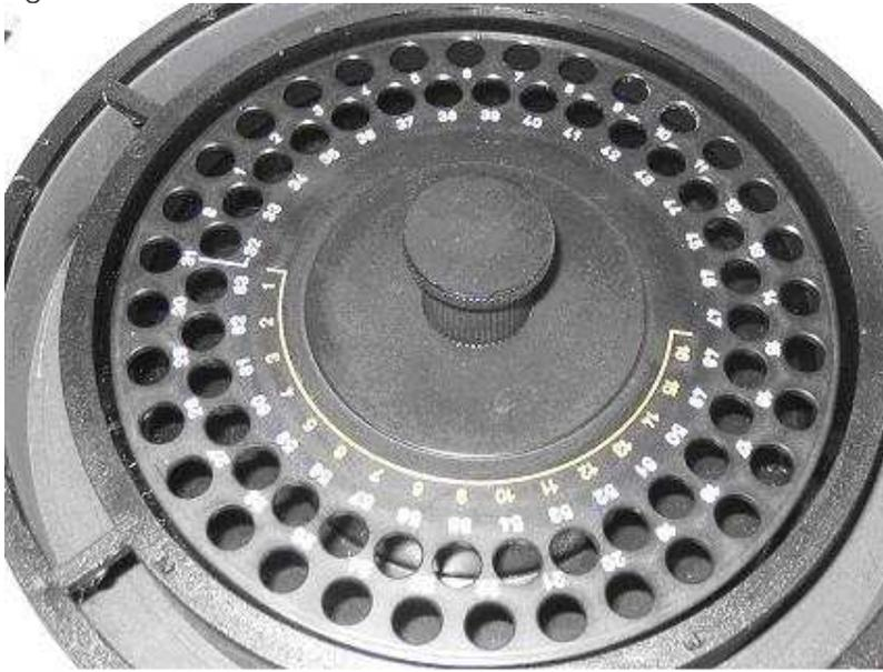
The INNER plate movement and position is controlled by a stepper motor driver (U6) located onboard to the Power board that drives the stepper motor model 23L-C304-76W and an optical sensor barrel that informs when the arm is at home position. The movement from the motor to the arm is transferred by a mechanism driven from a belt and two pulleys.
