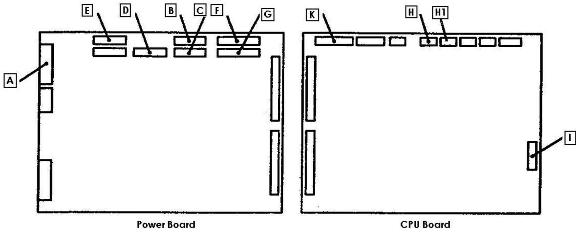
16) connect all the connectors of the cabling on the dispositives present on the instrument according to the following scheme:
