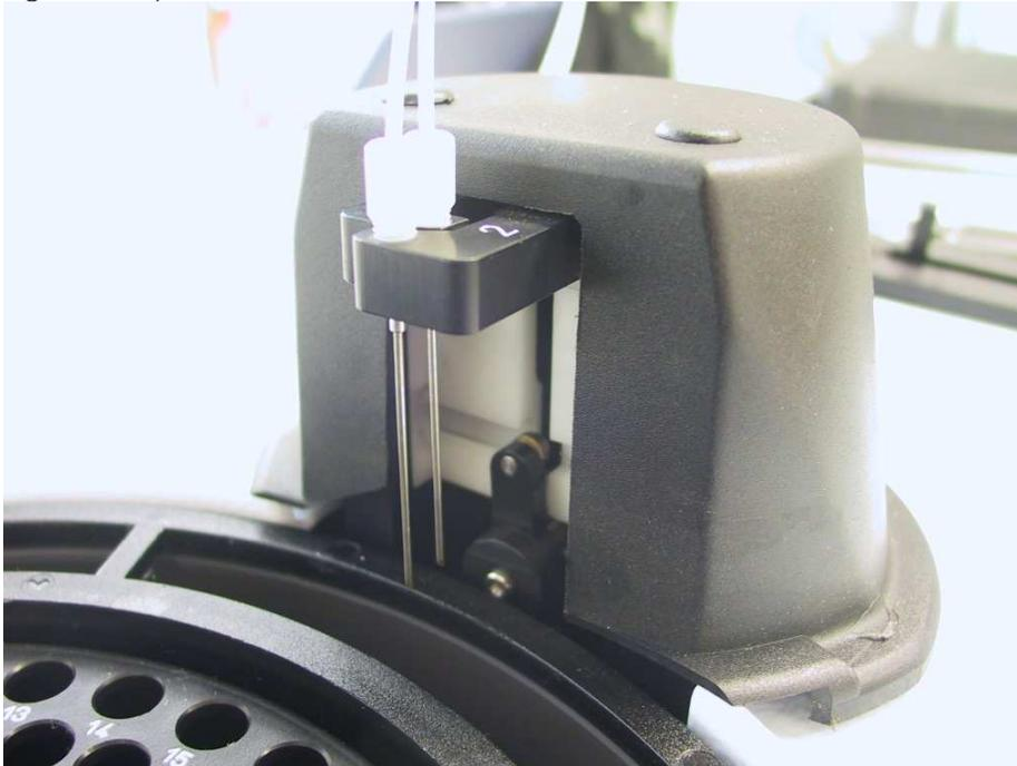
The ASPIRATION NEEDLE ARM movement and position is controlled by a stepper motor driver (U13) located onboard to the Power board that drives an stepper motor model 103-546-5342 ( for mono cuvette ) or an stepper motor model 103-547-52500 ( for double cuvette ) and an optical sensor barrel that informs when the arm is at home position.
