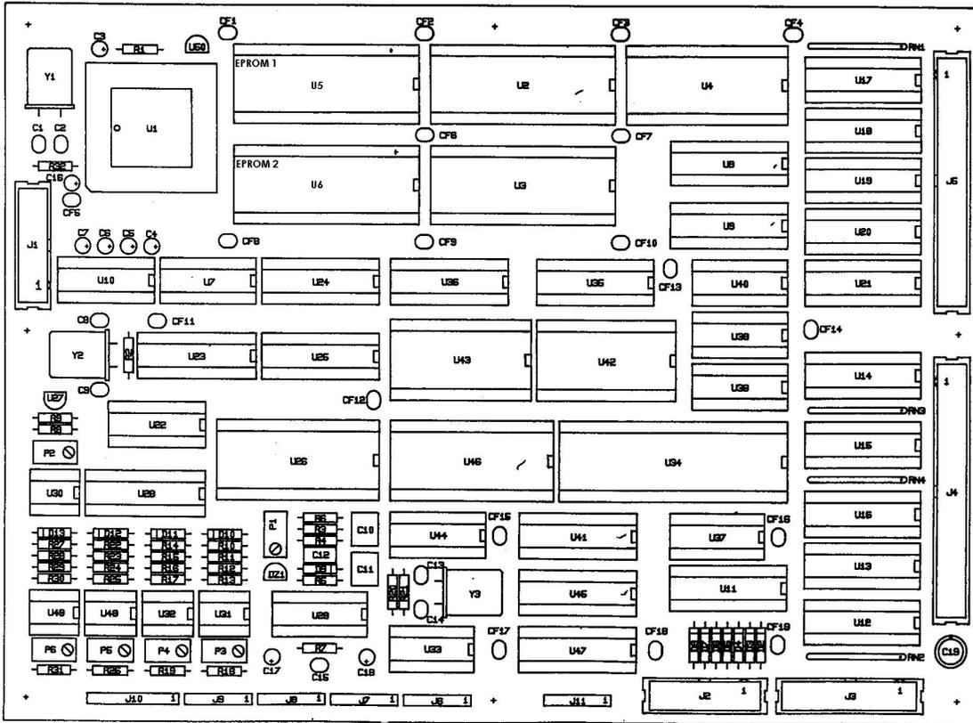
Figure 3 : Memory and Microprocessor
