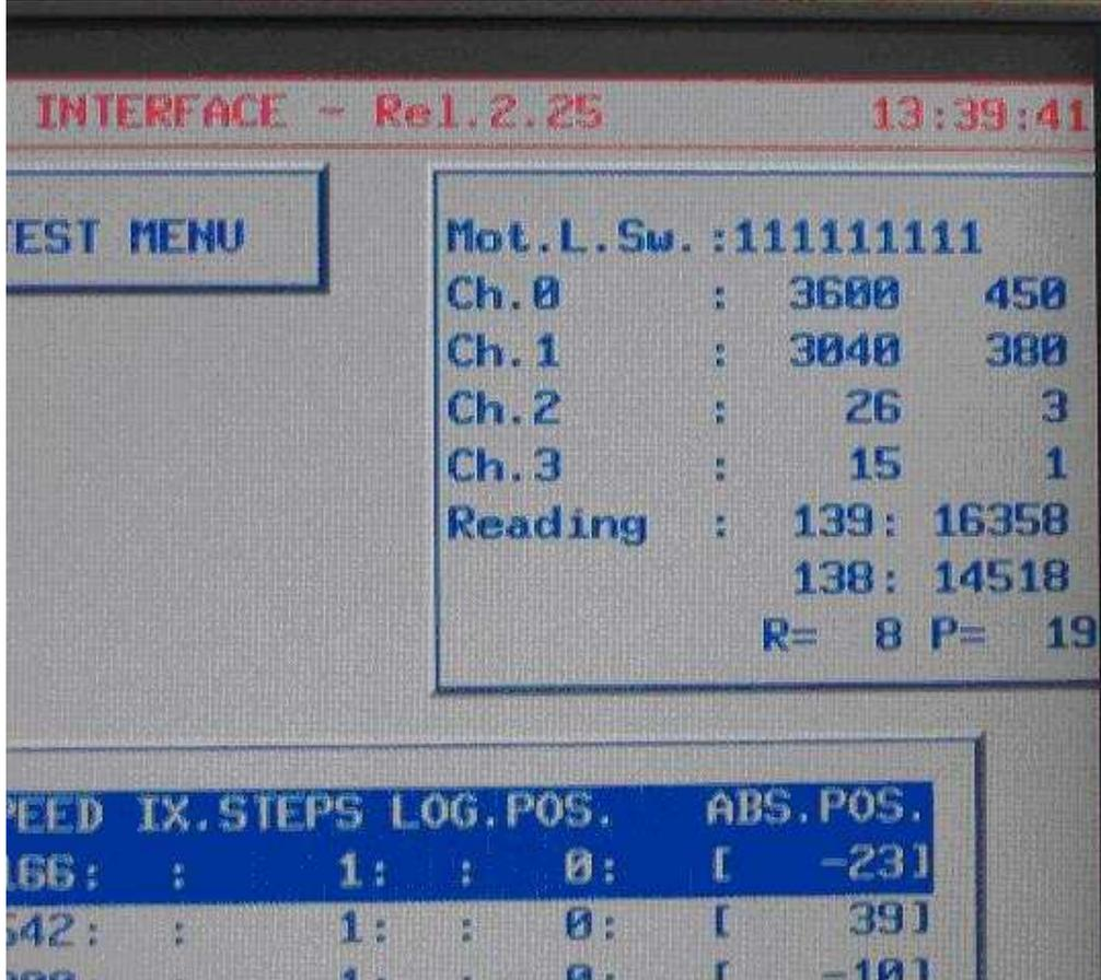
**MOT.L.SW.** : Indicates the logical status of the home position sensor and the logical status of the level sensor.
