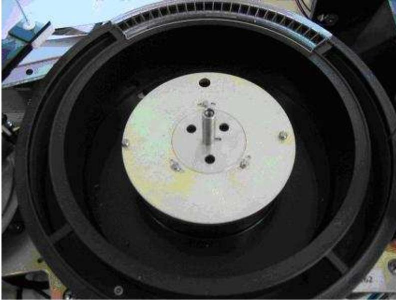
Figure 4: Outer plate ( double cuvette )
