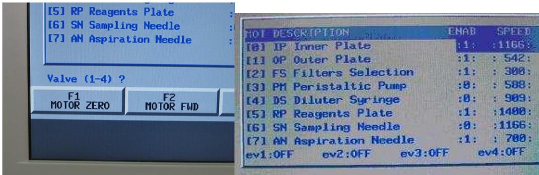
Select 3 and verify that the pump relative to the flow cell n°1 is moving in the clock wise direction.
