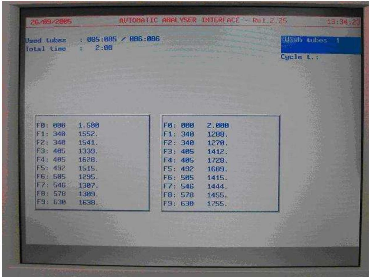
**F5 AUTOZERO** : Used to execute an autozero of the complete filter wheel.
