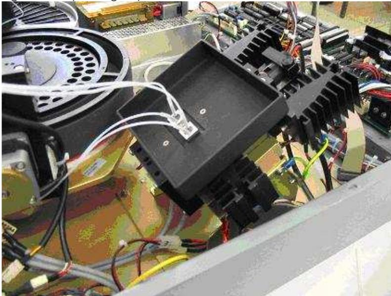
The FILTER WHEEL movement and position is controlled by a stepper motor driver (U8) located onboard to the Power board that drives an stepper motor model 23LM-C304-76W ( for mono cuvette ) or an stepper motor model 103-547-52500 ( for double cuvette ) and an optical sensor barrel that informs when the arm is at home position.
