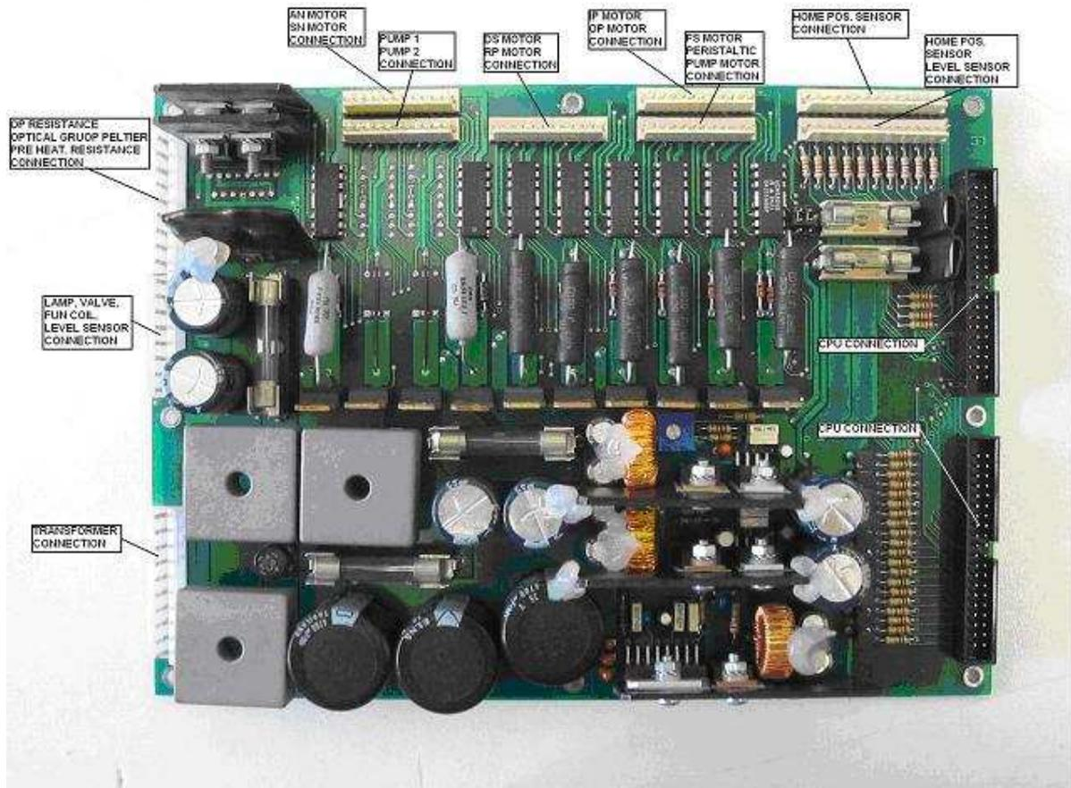
The POWER Board is the power interface between CPU and external devices like Stepper Motors, Home Position sensors, Temperature sensors and so on.
