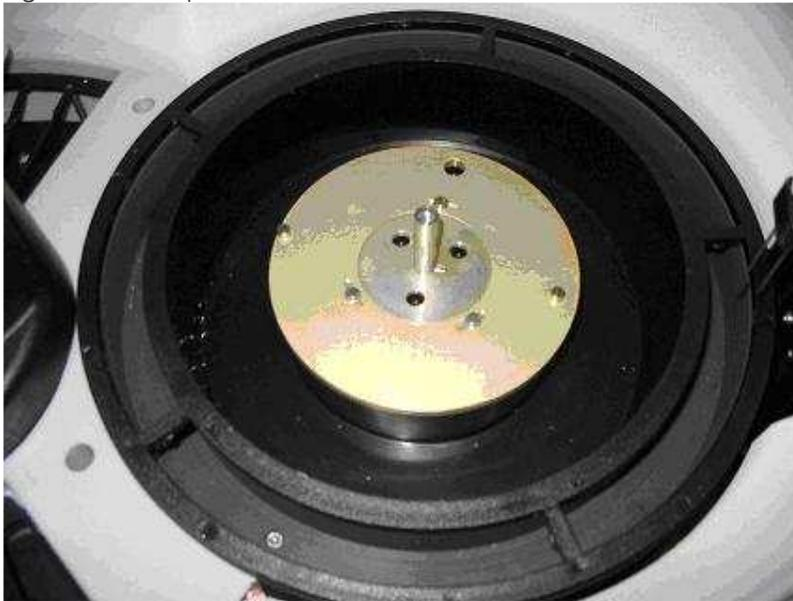
The OUTER plate movement and position is controlled by a stepper motor driver (U7) located onboard to the Power board that drives the stepper motor model 23L-C304-76W and an optical sensor barrel that informs when the arm is at home position. The movement from the motor to the arm is transferred by a mechanism driven from a belt and two pulleys.
