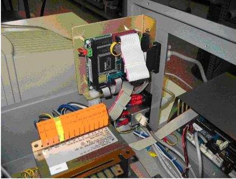
Figure 15: Cooling plate Power Switching + Motor driver Power Switching and Main Transformer
