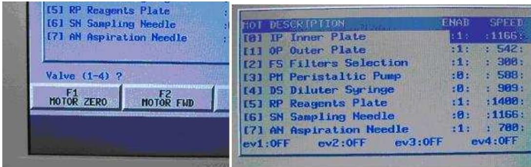
Select 1 and verify that the plastic cursor (black and white) present on the central part of the electrovalve of the diluter is moving correctly. At the end of this operation press another time 1 to leave the cursor in release position.
