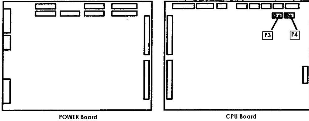
42) control the temperature indicated by the thermometer positioned into the false flow cell which should be of  $38,0\text{ }^{\circ}\text{C} \pm 0,2\text{ }^{\circ}\text{C}$ . Regulate the trimmer P4 of the CPU board rotating it in anticlockwise if the read temperature is inferior or in clockwise if it is superior.
