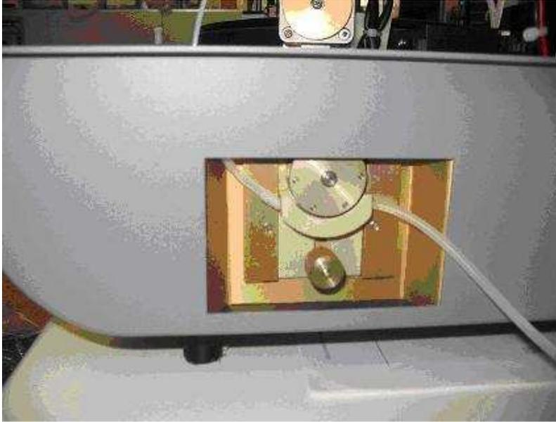
The PERISTALTIC PUMP movement is controlled by a stepper motor driver (U9) located onboard to the Power board that drives an stepper motor model 23LM-C304-76W. The movement from the motor to the rotor is direct.
